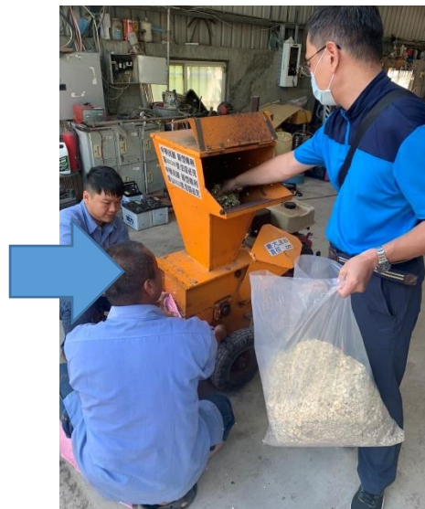
thorny bamboo coarse screening and cutting
