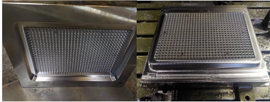
Figure 3. Thorny bamboo gardening board mold
